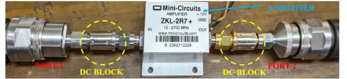
Fig. 6: Amplifier connection using DC-Block
