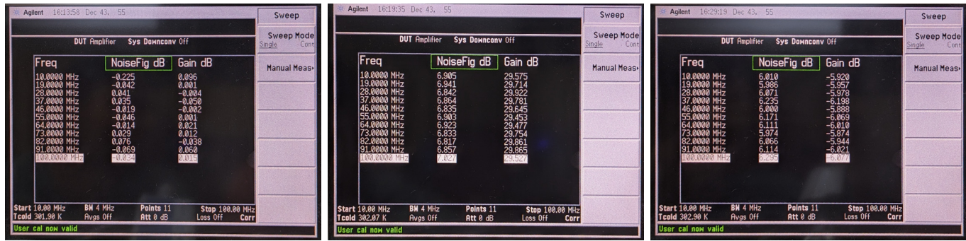
Fig. 3: Measurement results of Noise Figures for (a) a calibrated NF meter (b) an IF amplifier, and (c) an attenuator
